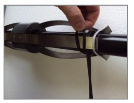
Ensure the short loop is in line with the release pin hole in the magnet body.
