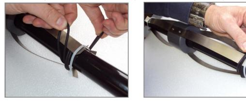
Wrap the long section of the rubber band over the spring legs and back to meet the short end.
