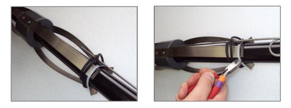
Insert the pin through both loops and through the hole in the magnet body.
