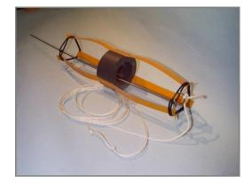
For installations where the spider magnets are to be individually installed by sliding over the preinstalled access tube and pushing down to their required installation level, the first spider magnet maybe fitted with its release pin or pneumatic cutters, but other than this, the instrument is ready for installation.
