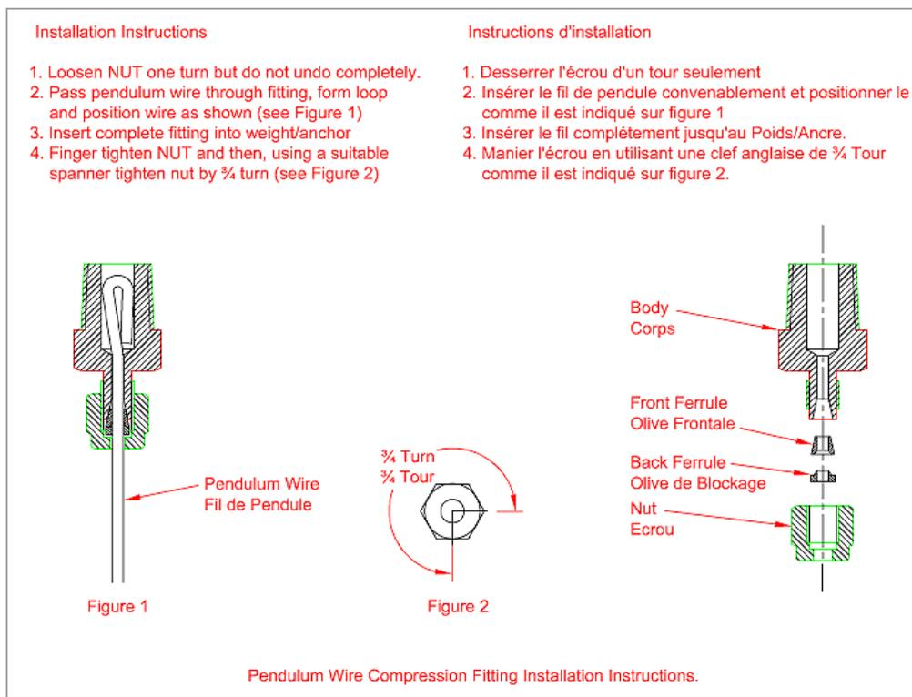
A suitable pull-test should be carried out to ensure that the wire is clamped correctly.
