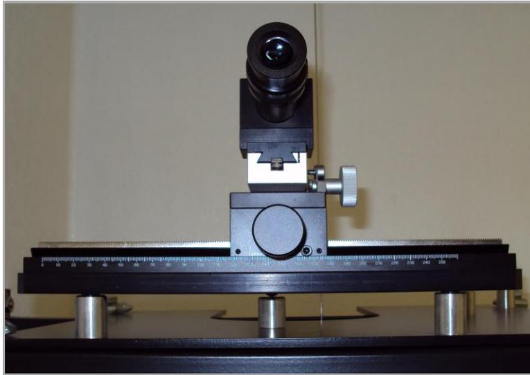
The co-ordinate position of the pendulum wire relative to the fixed reference frame is determined by adjusting the position of the microscope to view the edge of the wire against a graticule on the telescope lens. The control knob on the front of the microscope is used for traversing the microscope along the track. The control knob on the right hand side is used to focus the microscope on the wire by moving the microscope lens toward or away from the wire
