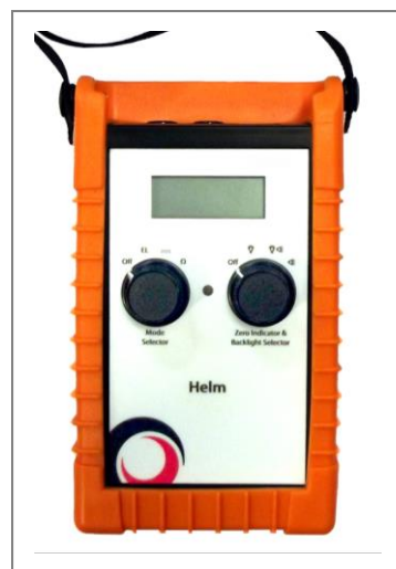
The HELM (Hand Held Electrolevel Meter); reads all Soil Instruments Electrolevel products, as well as up to 20VDC and 2K \Omega , making it an ideal readout for a variety of instruments as well as a tool to check power supplies and lead / sensor continuity
