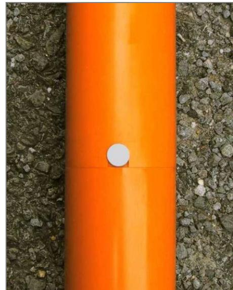
**WARNING:** DO NOT rock the upper casing backwards and forwards as this will distort the female section and damage the casing
