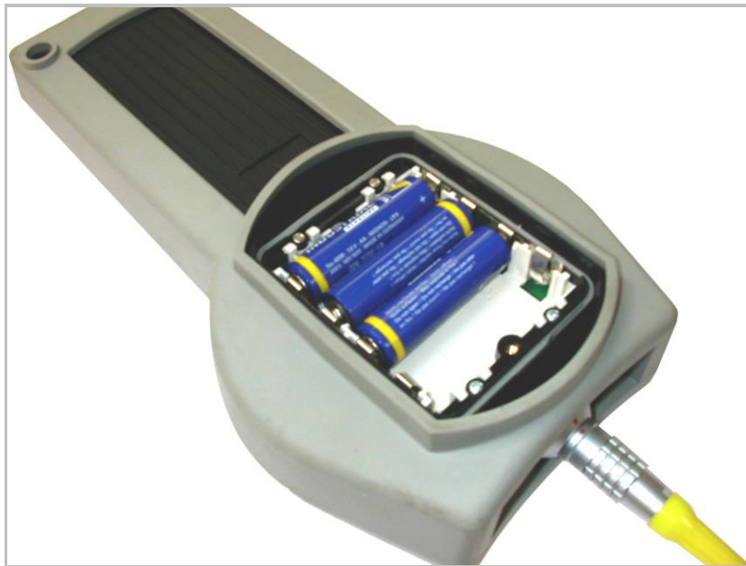
Battery compartment & flylead socket
