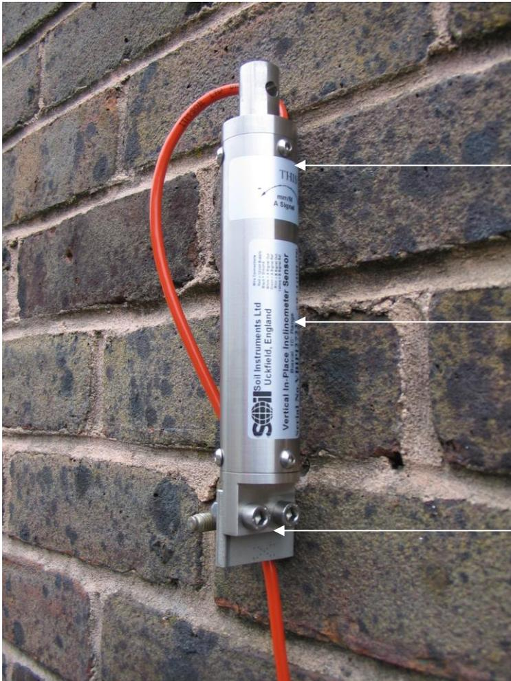
Label identifying sensitive axis – in the case pictured the wall is expected to move outwards so the sensitive axis is at 90° to the wall itself
