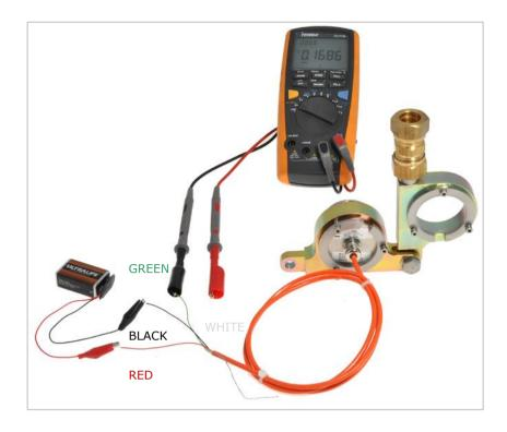
Alternatively use a Soil Instruments IPI Readout
