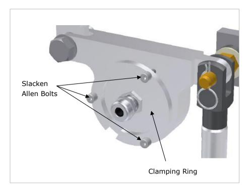
Adjust by rotating sensor housing until level ( $\pm 0.1$  volts). When viewed from the cable entry side (as above) an anti-clockwise rotation will cause a positive change in the mV reading.
