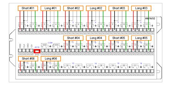
**NOTE:** For each sensor, drain wire for screen or shield should be connected to L1 terminal on AM16/32
