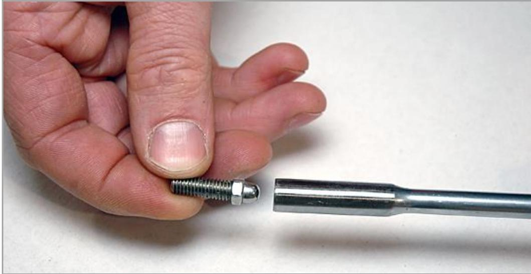
Tighten the reading datum fully into the rod connector and withdraw the nut spinner.
