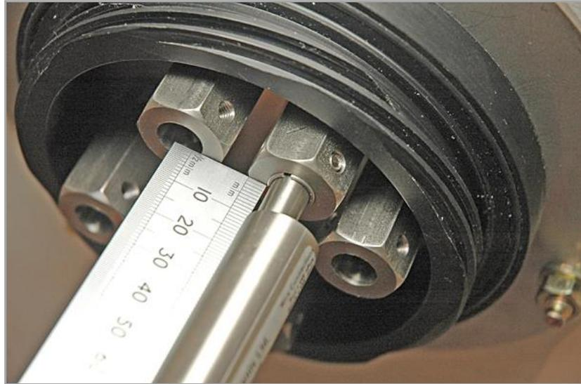
Install the remaining transducers and record the initial reading from each transducer, noting the serial number of the transducer and the hole position.
