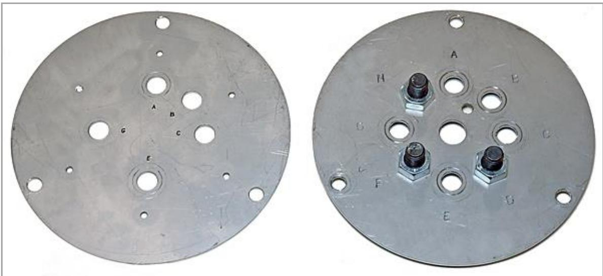
Position the grout plate centrally over the borehole and mark the plate fixing positions onto the mounting surface.
