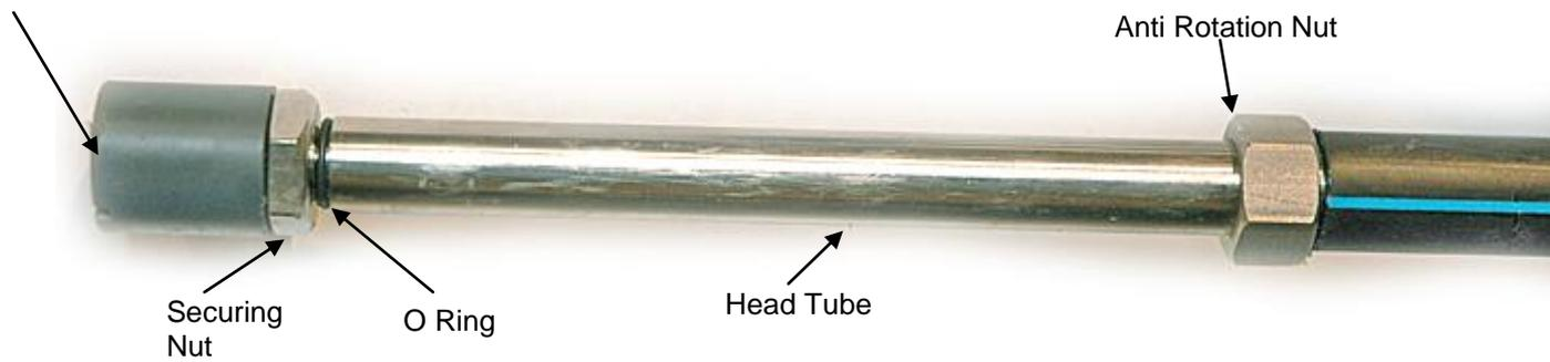
To fit the anchor head tube to the grout plate remove the protective cap and securing nut from the head tube and lubricate the "O" ring with silicon grease.
