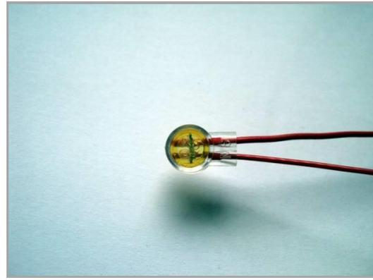
Test all connections after crimping to ensure continuity and security of connections.
