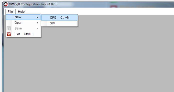
'Create Sections' allows you to choose the required sections. To create a new configuration file, enter the four digit serial number of the logger into the 'VWlog8 ID' textbox. This will create the name of the configuration file.
