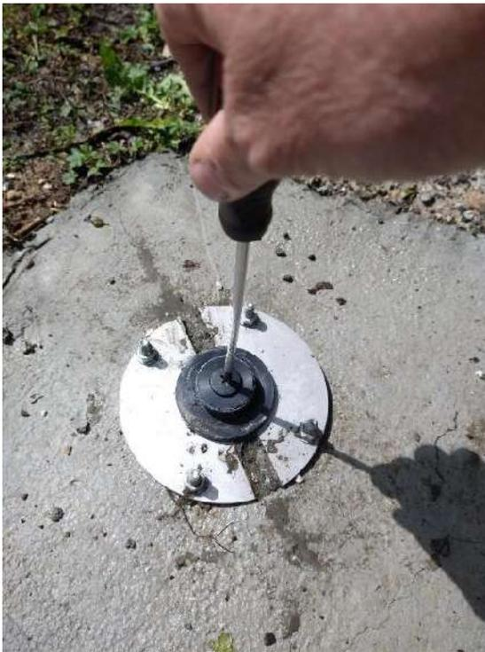
The checking of the zero setting should be performed before reading each borehole.
