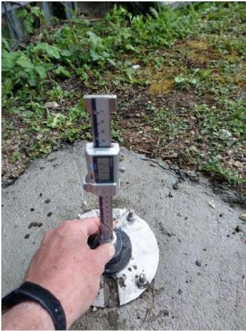
Slide the display towards the boss until the contact rests on the reading datum and record the reading that is shown on the display along with the anchor position.
