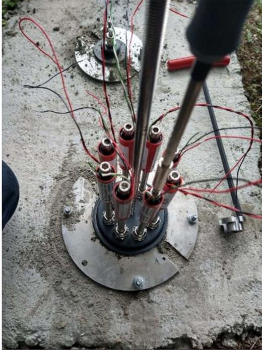
Do not over tighten, max 3 Nm
