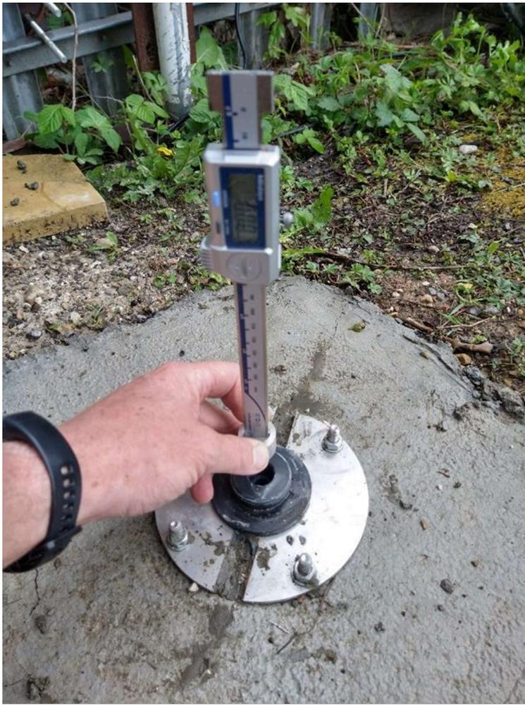
move the digital display towards the boss until the contact rests on the flat surface.
