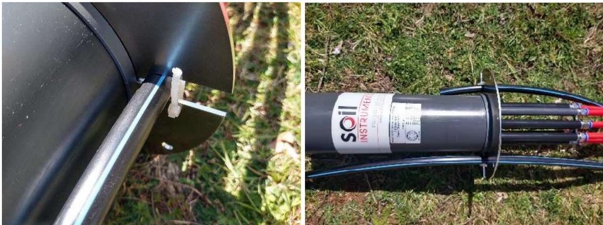
If the head is to be secured to a hard surface of rock or concrete the surface should be flat and perpendicular to the borehole.
