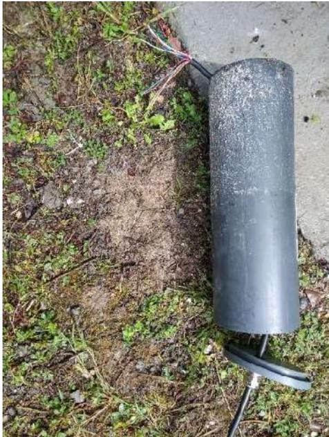
Cut off the ends of the transducer conductor wires so they are clean cut with no exposed copper conductor.
