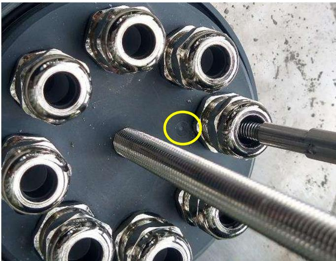
The other rods decrease in length in a clockwise direction around the head through to number eight, not all the positions will be populated with a securing gland depending on the specific configuration.
