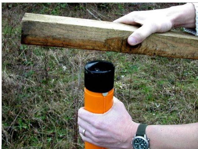
6. The casing should now be hammered down close to ground level. At this stage it may be necessary to extract the drill rods if you are not confident of assembling the rods inside of the inclinometer. Remove protective tape from 'male' end and offer the female end of the next length, ensuring that the keyways are aligned.
